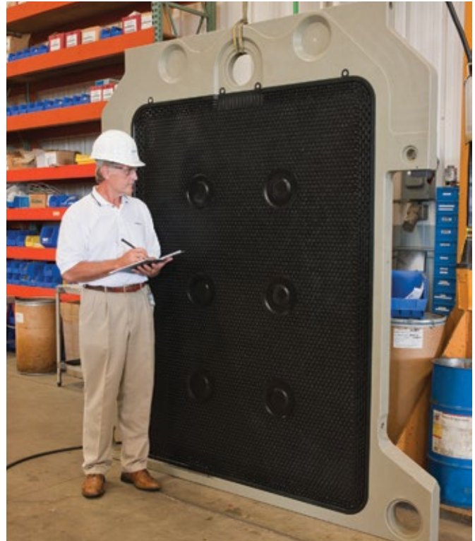
1.5 m x 2.0 m MC Press® membrane plates provide high capacity filtration
