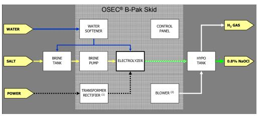
NOTE 1: FLOOR MOUNTED. TYPICALLY LOCATED ADJACENT TO SKID. NOTE 2: BLOWERS FOR CAPACITIES LARGER THEN 500 LB/DAY ARE NOT INCLUDED ON SKID ASSEMBLY.
