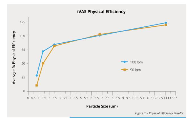
Due to the nature of a 0.8  $\mu$ m membrane filter sampler it can be assumed that it is 100 % efficient at all of the above particle sizes therefore, the d<sub>50</sub> value for the iVAS is the particle size at which the Physical Efficiency is 50 %. As can be seen from Figure 1 above this is around 1.1 µm when sampling at 100
