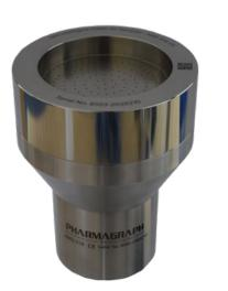
The Biological Efficiency testing showed that at both 100 lpm and 50 lpm the Biological Efficiency of the iVAS was greater than that of the Casella reference sampler.
