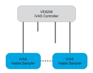
A single cable carries both RS485 communications and 24Vdc power to each iVAS. The connection is via a quick release connector on the free-standing pedestal unit or via a cable rising through the mounting column in the tri-clamp variant. This ensures fast and straightforward iVAS swap outs.
